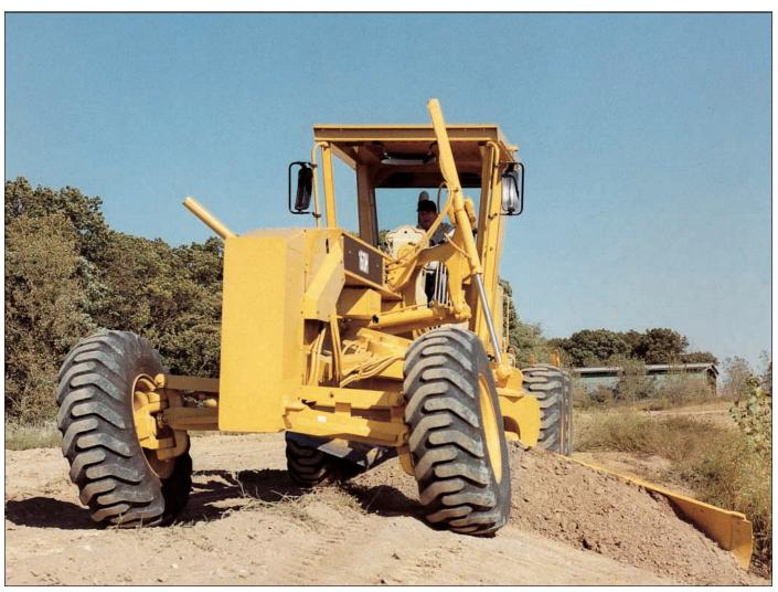
**Blade positioning.** The blade linkage design enhances moldboard positioning. This blade linkage is most beneficial in ditch cutting and cleaning.
